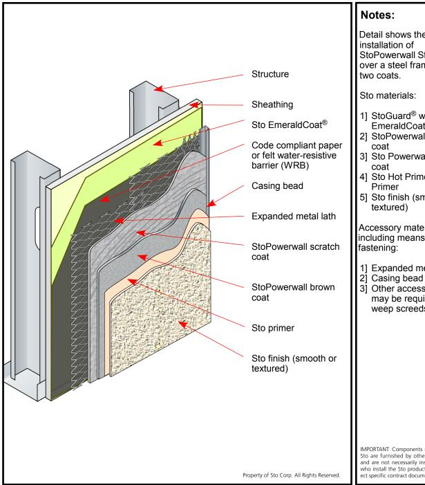
Detail shows the StoPowerwall Stucco over a steel frame wall in
